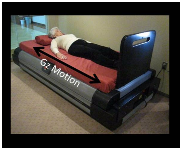
Figure 1. A subject lying on the motorized platform that delivers Whole Body Periodic Acceleration (WBPA). The footboard fixes the feet with shoes onto it to prevent slippage while the platform is moving.
