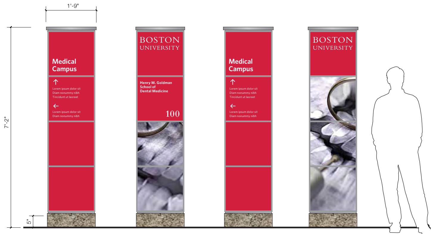
A: Directional Panel B: College/School ID C: Directional Panel D: Image Panel 1/2" = 1' - 0"
