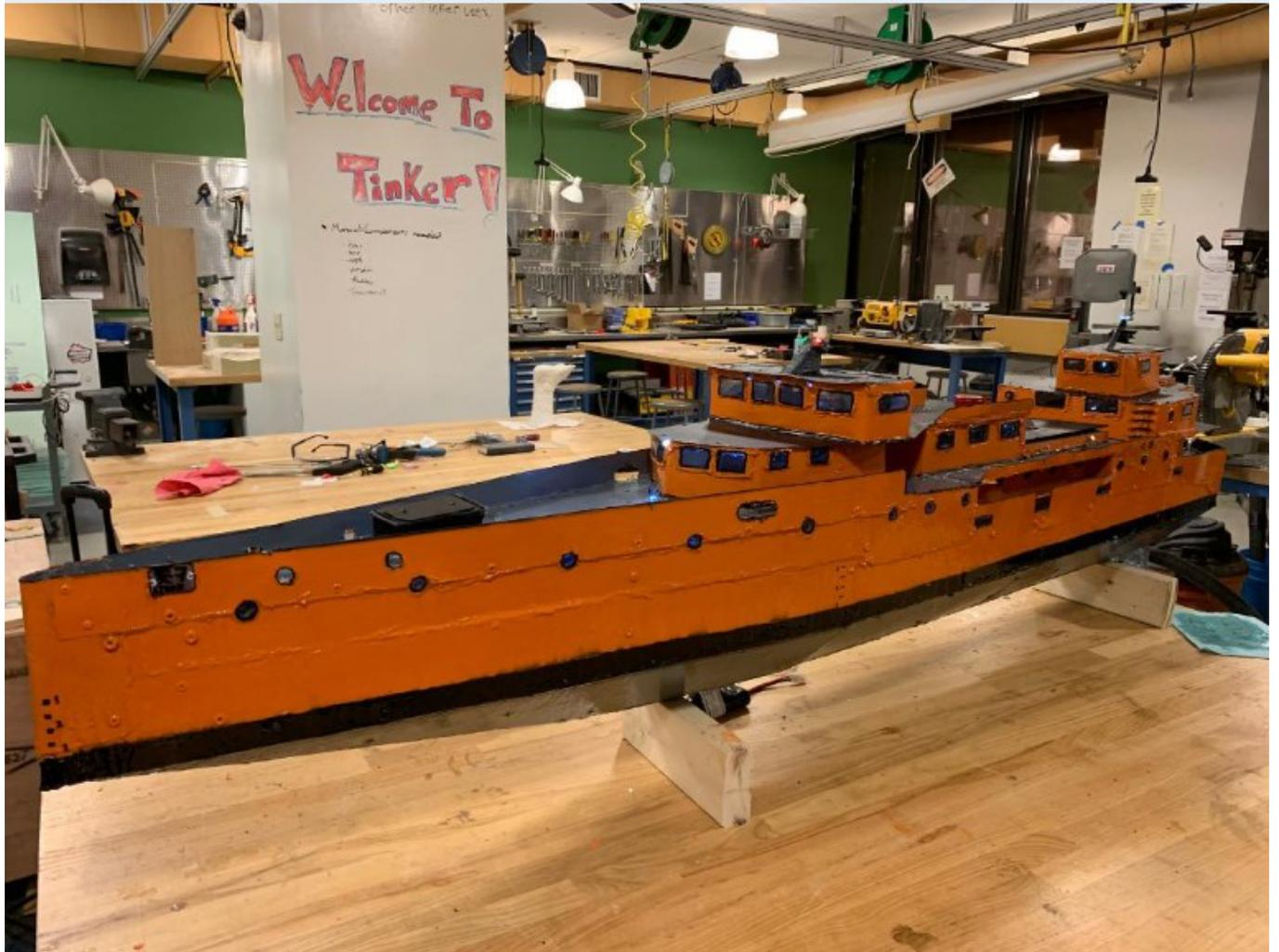
I finished painting the ship, then ensured that all cracks were caulked or hot glued. Then the entire ship was coated with epoxy to eliminate any remaining cracks.
