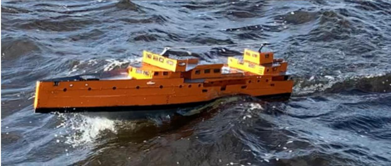
I took the ship to the Charles River with a strong wind creating ~6 in. average waves. The motor provided plenty of power for navigation upwind. Cross-sea performance is quite good with the roll dampers. Downwind performance is stable in all axes also. Upwind, in certain wave conditions, the ship will resonate in pitch. By observing videos of full-scale ships in similar conditions, this seems to be an expected effect.
