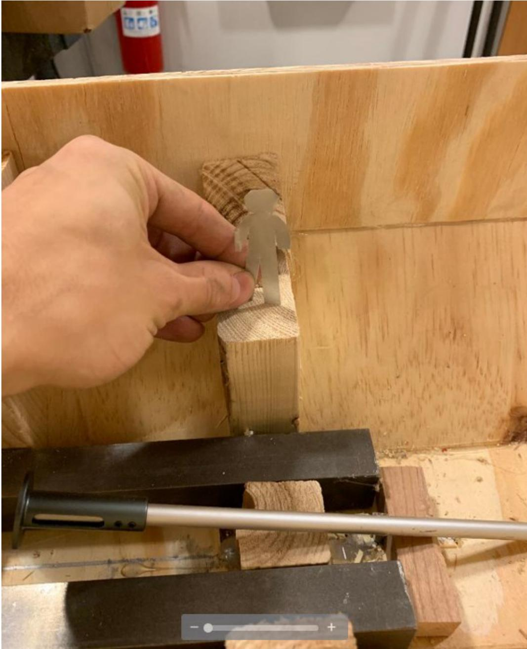
The figure that I am holding in the picture is equivalent to a 6 ft. tall person. Instead of scaling an actual boat down and building a model, these ships are of my own design. Therefore, I use the scale figures to build features that a 1/32 scale crew could use. Also visible are two of the steel bars used to ballast the ship. There are probably 40-50 pounds of ballast in the bilge of the ship.
