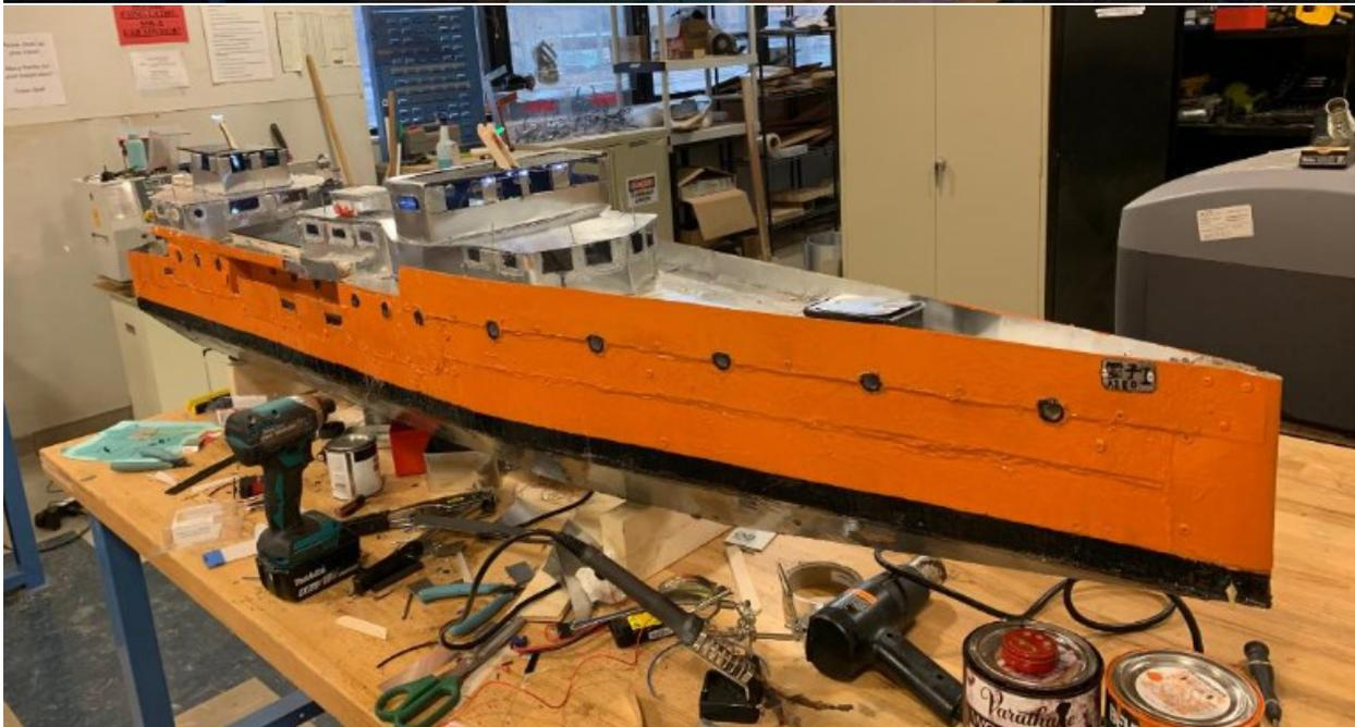
I continued building the superstructure and installing lights. There are two new lighting circuits. One powers most of the main deck lights as well as some of the crew quarters and the upper forward decks. The other illuminates the rest of the upper decks and powers the navigation lights. Note that the nav lights are backwards in this picture due to distracted gluing. This was subsequently fixed.
