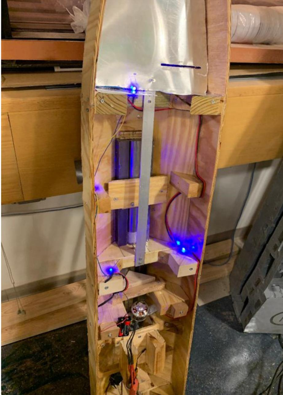
I began adding the deck for the first belowdeck level (second belowdeck level is the bilge where the ballast and sewage tanks are). I also began adding lighting. These are blue LEDs soldered in parallel and connected to two AAA batteries and a switch with a resistor.
