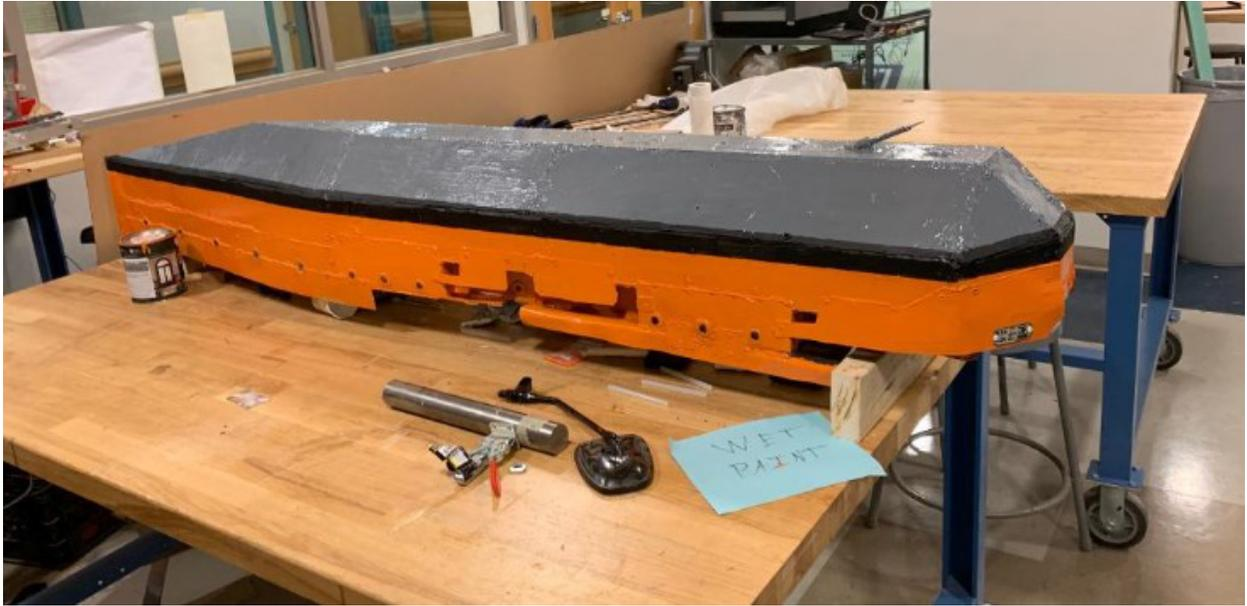
At this point, the ship was turned upside down and the outer hull was coated with epoxy. Once the epoxy cured, the hull was painted, then coated with more epoxy. I also made name plates.
