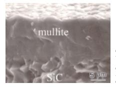
A scanning electron microscope image of a 10micron-thick environmental barrier coating on silicon carbide.
