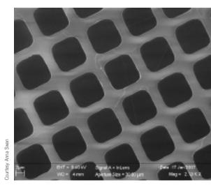
Scanning electron microscopy image of carbon nanotubes grown across voids 7 micrometers across.
