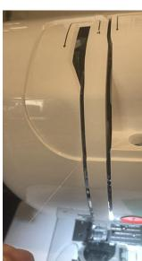
For step 5, pull more thread out to both confirm that it didn't get snagged anywhere and so that you have enough extra for the needle threading action.
