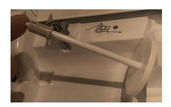
Put it on so that the 3 pronged end is facing the open end of the spool pin and push it as far down the pin as it will go.
