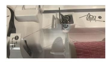
For step 4, pull the thread to the right until you have about 3 in or 9 cm of thread that goes beyond the edge of the body of the sewing machine.
