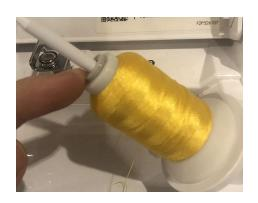
Once the spool and spool insert are on the pin, the last step in loading the spool is to put a spool cap on the end of the pin. This helps hold everything in place and helps make sure the thread unspools at an even pace and without getting tangled. The spool cap needs to be at least as large as the end of the spool, in this case the smallest of the spool caps is large enough.
