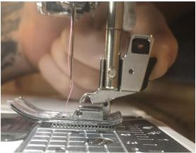
Carefully pull the foot out from the needle area.
