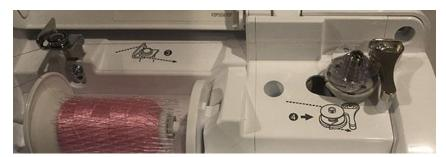
Take this thread and slide it under the clear plastic of the bobbin shell.
