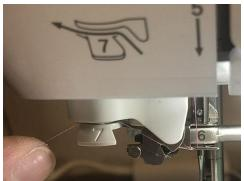
Then pull the thread further to the left and up on the side of the machine is a protected blade that you can use to cut any excess thread.
