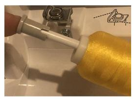
Put it on so that the 3 pronged end is facing the spool and push it all the way down until only the lip of it is showing at the top of the spool.
