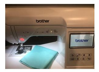
Once you tap the touch screen to fully wake the sewing machine up, the needle will shift left/right until it is in position to sew the first stitch in its menu.
