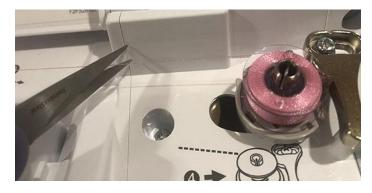
Then pull the bobbin mechanism back to the left and pull the bobbin up and off of the pin.
