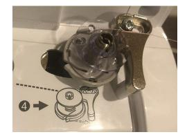
Then wind it clockwise and tightly around the middle of the bobbin 4-6 times.
