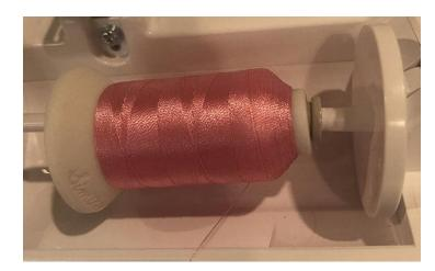
Once the spool insert and spool are on the pin, the last step in loading the spool is to put a spool cap on the end of the pin. This helps hold everything in place and helps make sure the thread unspools at an even pace and without getting tangled. The spool cap needs to be at least as large as the end of the spool, in this case the largest spool cap is the best fit.
