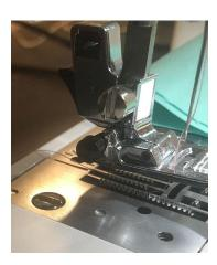
At this point the spool thread is fully set up and you can close the top cover of the machine if you wish. Leave the safety button pressed, you will still need the needle stopped for putting the full bobbin in the machine.
