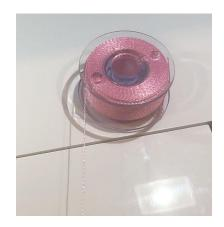
Drop the bobbin into the main opening in the machine.
