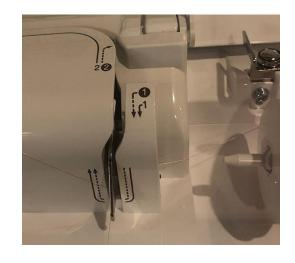
For step 2, bring the thread to the left, going through the curved slot in the machine.
