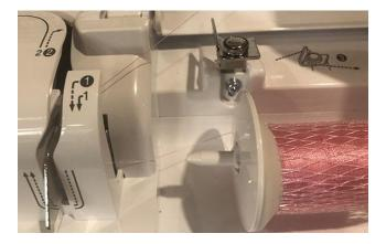
Step 3 will be loading the thread around the tension setting disc for bobbin winding. This is one of the most important steps in bobbin winding as it makes sure that the thread is tightly and evenly wound on the bobbin.
