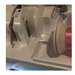
Hook the thread under the metal guide and bring the thread up so it is sandwiched between the metal and plastic on this side as well.
