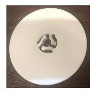
The spool cap should go on so that the concave part is facing the spool. It should be pushed as far down as possible so that there isn't room for the thread to get between it and the spool insert when it is unwinding.
