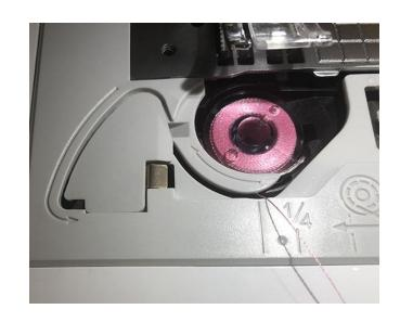
Bring the thread through the slot, following the full curve to the end.
