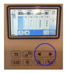
When you find the stitch you want, tap it on the screen so it is highlighted in blue. The needle may shift so it is positioned correctly for the stitch.
