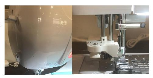
After the needle is threaded, the mechanism will pop back up and you can slowly raise the lever back to the top of the machine. You can also raise the foot again at this point.
