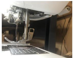
Just above the back of the foot itself, there is a small black lever. Push this in to unlock the foot, it should drop on its own after the lever is pressed.
