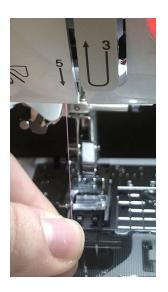
In step 6, push the thread behind the arm below the #6 on the machine. Then pull towards the left to pull the thread into the eye of the arm/post. This will help guide the thread into the eye of the needle as the machine is running.
