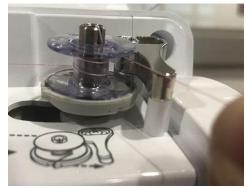
After winding it several times, take whatever thread is left and guide it through the slot in the gray plastic under the bobbin base. Pull the thread to the right until it is tight and seems unlikely to shift.
