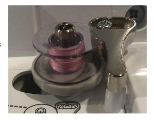
If you are planning on sewing a full garment or doing a lot of embroidery, you may want to fill the bobbin completely. In this case, let the machine run until it starts to slow down or until the thread starts to hit the metal arm to the right of the bobbin. Once either of these happen, press the start/stop button again to stop the machine.
