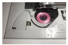
At the end of the slot is a small blade, pull the thread against it to cut the extra thread off if you are going to let the machine grab the bobbin thread automatically. In most cases, this is what you want to do.
