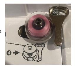
Once it has stopped spinning, cut the thread connecting the bobbin to the spool. I recommend cutting so there is a 2 in or 5 cm tail of thread coming off the bobbin.
