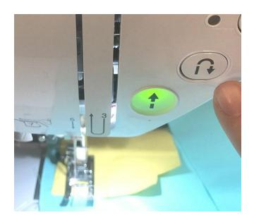
After the machine stops, press the scissor button on the front of the machine to cut the extra thread tails and raise the needle out of your fabric.
