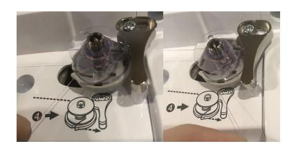
Then cut the excess thread close to the underside of the base to prevent it from tangling under the bobbin area.
