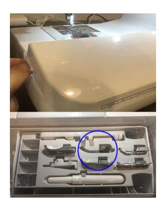
If you need to change the foot, the first thing you need to do is press the safety button on the front of the machine to lock the machine.
