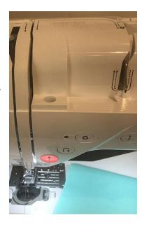
In step 3, pull the thread back up and to the left, hooking it around the curved plastic at the base between the two vertical slots in the machine. Pull the thread all the way up.
