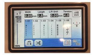
Once you have your stitch selected, you will need to confirm that the foot installed in the machine matches the foot that the stitch requires. The foot the stitch wants you to use will be displayed in the upper left hand corner of the touch screen, just above the line showing what the stitch will look like.
