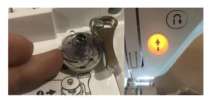
Next, you follow the numbered arrows with the dotted lines guiding the thread from the spool to the bobbin.
