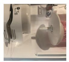
Hook the thread under the metal guide and bring the thread up so it is sandwiched between the metal and plastic on this side as well.
