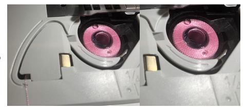
After cutting the thread, replace the clear cover over the bobbin area. Line up the end with the hole in the case and push it in and down until it clicks.
