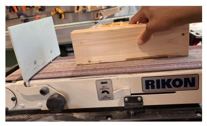
I then used the belt sander shown to the left, to smooth off rough edges or corners. An optional step is to save chips or sanded off material in a paper cup, as it can act as a filler for any cracks in the wood!
