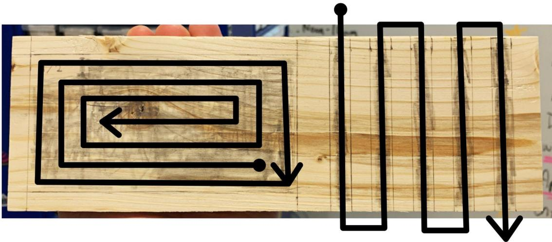
Line up the end mill with the slot markings you made and start milling at the correct depth along the path from the outside of your piece all the way through to the other end. As you start approaching the edge of the other side of your piece, move the end mill more slowly to lower the chances of splintering the wood as the mill exits your piece.
