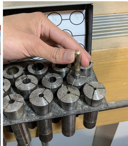
Afterwards, grab a collar from inside of the top drawer of the red tool cabinet. Unscrew the threaded part and slide it over the bottom of the collet moving it towards the top. Make sure that the threads are facing the top of the collet when you put the threaded part on. Screw the top of the collar onto the threaded part and tighten it by hand.
