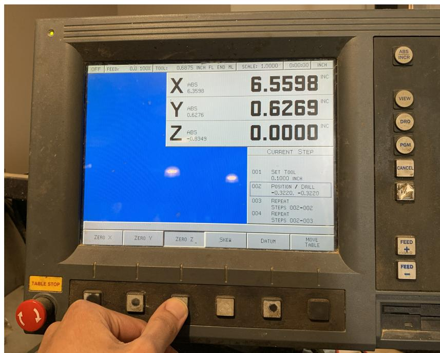
Before milling, ensure that the end mill rpm is set to around 1300-1400 rpm. DO NOT ADJUST THE RPM WITHOUT TURNING THE MILL ON FIRST.
