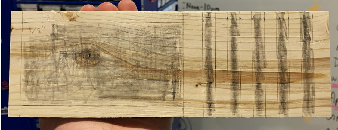
7. Use the NC mill with a  $\frac{3}{8}$  inch end mill to create the slots and compartment of the desk organizer.
