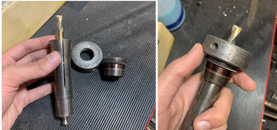
After that, place the tool into the tool holder at the corner of the NC mill closest to the red tool cabinet. Use the wrench in the top drawer of that cabinet to tighten down the collar onto the collet as much as possible. You can now insert the tool into the NC mill. **Ask a lab advisor to verify that you have done this correctly.**
