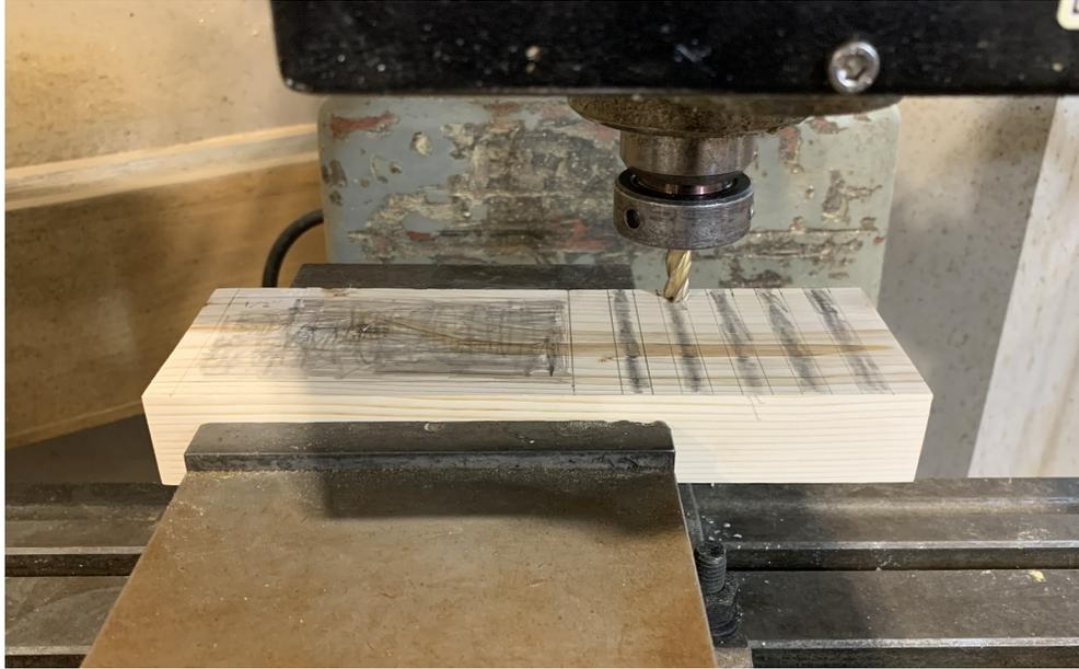
To ensure that you mill at the correct depth, lower the end mill **with the machine off** down to your piece so that the tip of the end mill touches its top face. Afterwards, zero the Z-axis on the digital display of the NC mill by pressing the third gray button from the left below the display.
