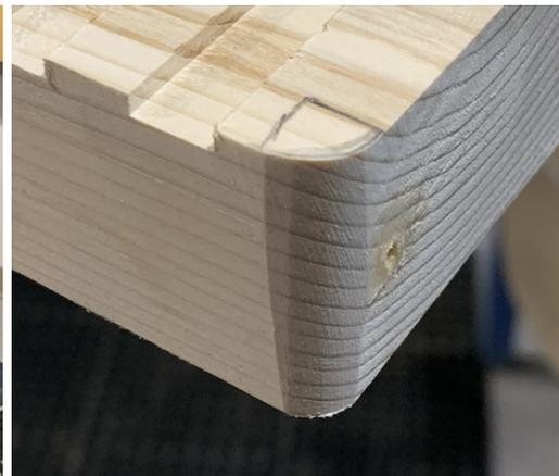
10. Use the router with a rounding over bit to round the base edges of the desk organizer. I recommend using a  $\frac{3}{8}$  inch bit, but you can use a  $\frac{1}{2}$  inch bit or other bit of your choice. Use clamps to ensure that your piece does not move while rounding the edges. The router bit should only stick out about as far as shown in the picture below:
