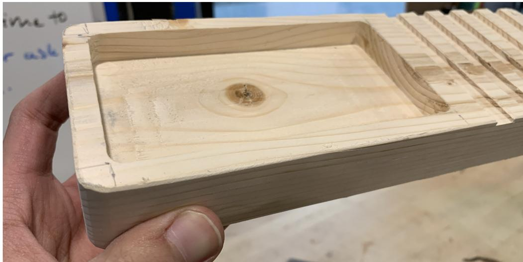
12. Finish off by sanding any unsanded parts of the desk organizer. For the inner faces of the compartment, you can use a small sheet of P150 sandpaper from inside the large blue cabinet near the stock area and sand them by hand.
