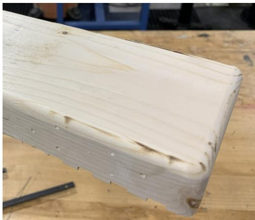
11. Use a hand file to make a small chamfer along all the top edges of the desk organizer except for the edges at the top inside edge of the large compartment.
