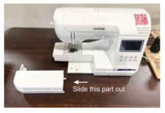
b. Open the channel for embroidery unit connection that is on the side of the machine.
