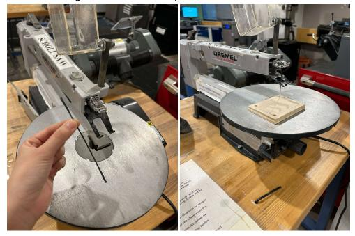
9. Adjust the foot to be just above the wood to give it support. Use the Allen key by the scroll saw to loosen the screw on the side. Adjust the height of the foot, then tighten the screw. Make sure the guard is down.
