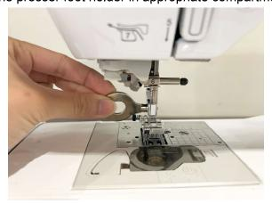
f. Put the embroidery foot in. Orient the foot appropriately then tighten the same screw to hold it using the screwdriver.
