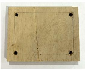
**8.** Ask SILab advisors for help with this step. Remove the scroll saw blade and insert it into one of the drilled holes. Put the blade back in the machine. Position the wood so the blade will cut along the line drawn in step 6.
