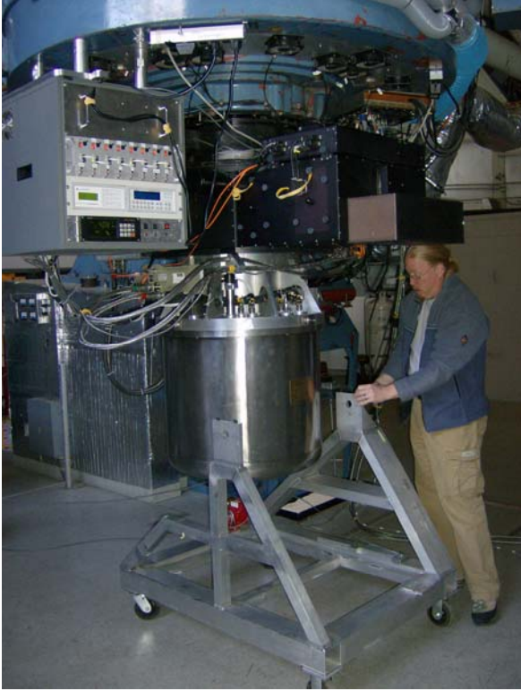
Brian Taylor completing installation of Mimir on the Perkins Telescope. The carrier cart is being wheeled away from the stainless steel cryostat; the electronics box is mounted in the upper left. The two metallic cables leaving the cryostat below the electronics are high-pressure helium lines that are part of the closed-cycle refrigeration system that keeps the optics and detector cold.
