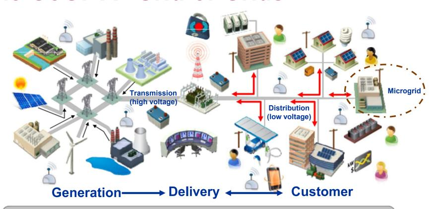
An Interconnected Power System Balancing Forecasted Resources with Dispatchable Loads
