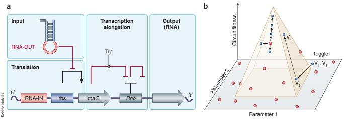
Figure 1 | Modularity improves design in synthetic biology. (a) A system to convert regulation of translational initiation into regulation of transcriptional elongation<sup>1</sup>. (b) Plug-and-play part replacement (black arrows) can optimize the performance of circuits designed discretely (blue dots) or combinatorially (red dots).
