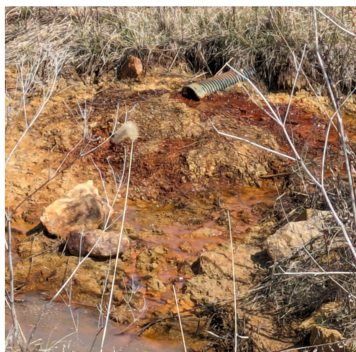
Figure 2: Red soil color near water sources indicates the presence of iron oxide as a result of pyrite oxidation.
