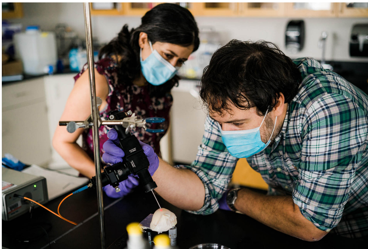
Michael Albro (right), an ENG assistant professor of mechanical engineering, and postdoctoral researcher Masumeh Kazemi using the Raman needle probe on an excised bovine cartilage specimen.
